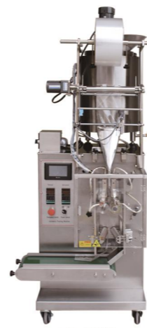
LD-240L Liquid automatic packaging machine
