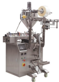
LD-320AB/LD-380C Fully automatic packaging machine with volumetric cups and chain-type volumetric batchers
